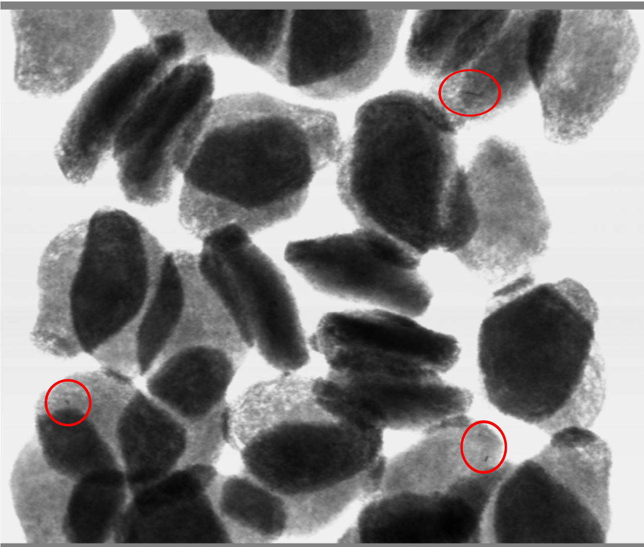
Figure 1: Tiny bits of bones are visible and have been circled with red rings in the image. No “artificial” bones have been added, the detected bones are in the product
