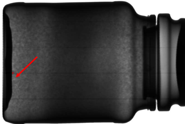
Fig. 2. Less than 2 mm glass piece detected using the novel high sensitivity technology. Note the position of the glass piece close to the bottom
