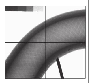
For extruded products such as rubber hoses, the typical performance is the detection of particles down to 0.5 mm in diameter in hoses with wall thickness of up to 1.5 mm, at line speed of 30 m/min. At the same conditions, holes are detected with diameters from 0.3 mm. Typical false reject rate is less than 0.5 percent, or less than 0.5 meter false reject for 100 meter hose.
