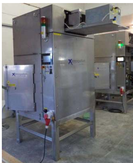
InnospeXion may provide the shutter system integrated with tailored X-ray cabinet, high stability X-ray source, control system, user interface, and mechanical mounting parts
