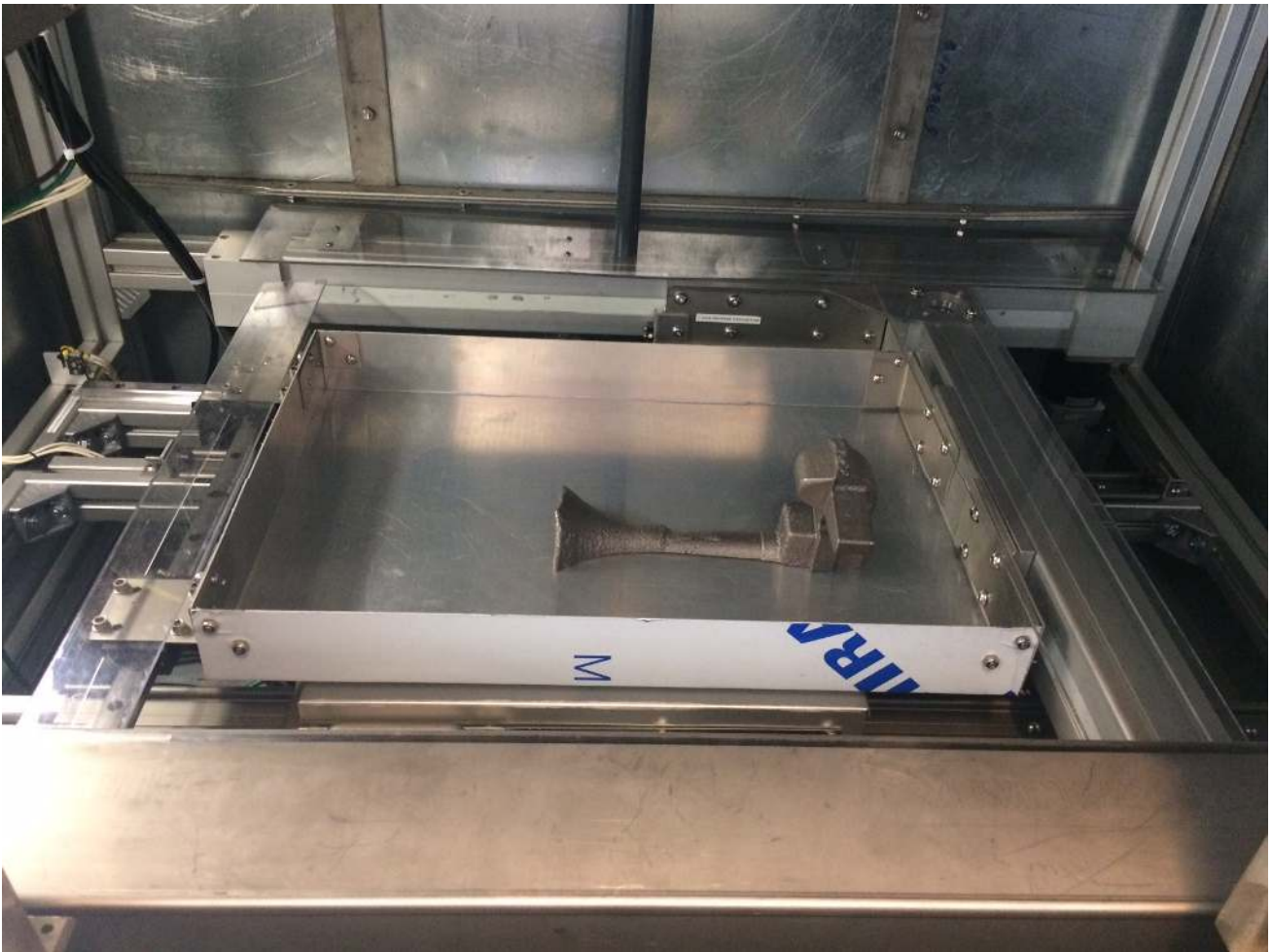
Fig. 3. Samples are positioned on a tray and scanned according to a pre-defined scan sequence programmed into the system master PLC.
