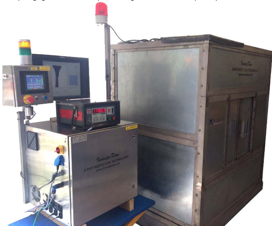
Fig. 2. The cast iron X-ray inspection system: High energy X-ray imaging up to 300 kV for revelation of defects in sand cast iron samples for high performance usage
