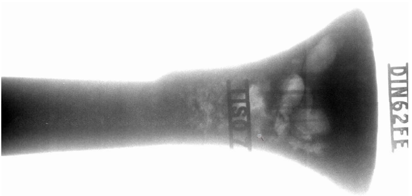
Fig. 1. X-ray imaging of a cast iron sample, showing abundant voids and porosity.
