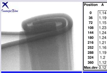
X-ray image acquired through a can seam. using the tangential imaging technique of the can under rotation. The can may be inspected and the seam assessed continuously during an entire revolution.
