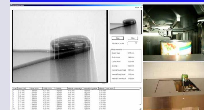
The user interface is simple, reflecting that the system is completely automatic. The can seam measurements are performed without any operator decision taking, is accurate and reproducible. All data are stored according is sensed. The entire sequence last < to the customer specific requests.
