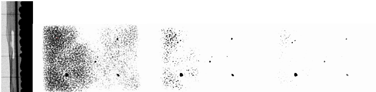
Figure 4: The contrast of the images can be adjusted according to the level of detail desired. Even the plastic bag is visible at 18kV (But not at 25kV – it is too thin to stop a 25kV X-ray).
