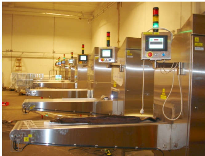
Fig. 1. X-ray systems for fur quality sorting during initial testing
