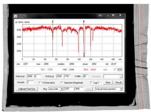
A typical scenario for product packed in pouches: folds in the seal zone (at the right side) may cause leaks or weak points where a product leak may arise with handling and/or time. The red lines at the right are taken across the seal. Deviations from a uniform level (here around 2450 GV's) denotes folds or leaks. Upon scanning, these zones are automatically detected and the pouch is sorted according to the criticality of the deviation identified by the system.
