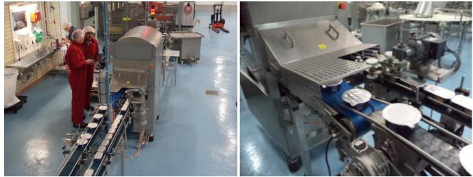
An automatic X-ray seal inspection system installed on a dual conveyor line, with plastic can products running 150 and 120 cpm. The can sealing is verified with a total reject rate of around 1 per cent, of which product irregularities constitute the vast part. Real seal errors (product in seal) is typically < 0.2-0.4%.
