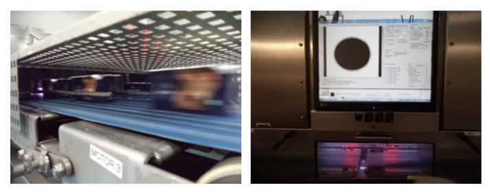
The **seal integrity assessment systems** are a variety of the "HYMCIS" products, which have been on the market since 2006. The applications range from raw material quality control and sorting, to fish and chicken bone detection and rejecting, in real time.
