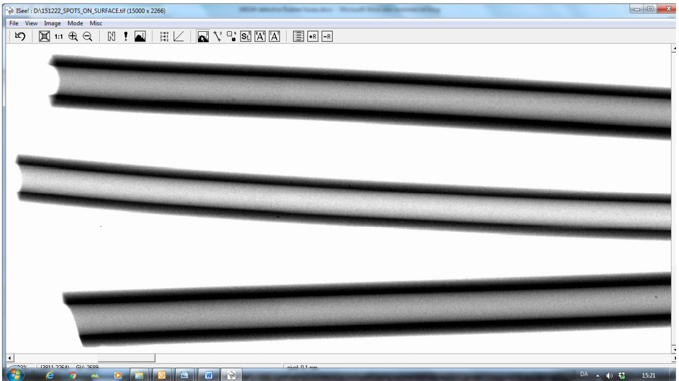
Bottom 3 hoses – leftmost part – these hoses are thicker than the others.
