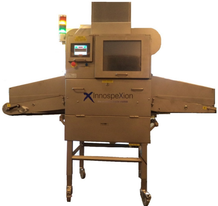
Fig. 3. Lobster entering X-ray system tail first. Fig. 4. The InnospeXion Lobster/Crustacean grading system is based on significant experience in providing fish bone detection system suitable for the harsh environment in the lobster processing industry.
