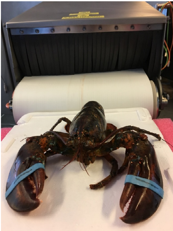
Fig. 3. Lobster entering X-ray system tail first. Fig. 4. The InnospeXion Lobster/Crustacean grading system is based on significant experience in providing fish bone detection system suitable for the harsh environment in the lobster processing industry.
