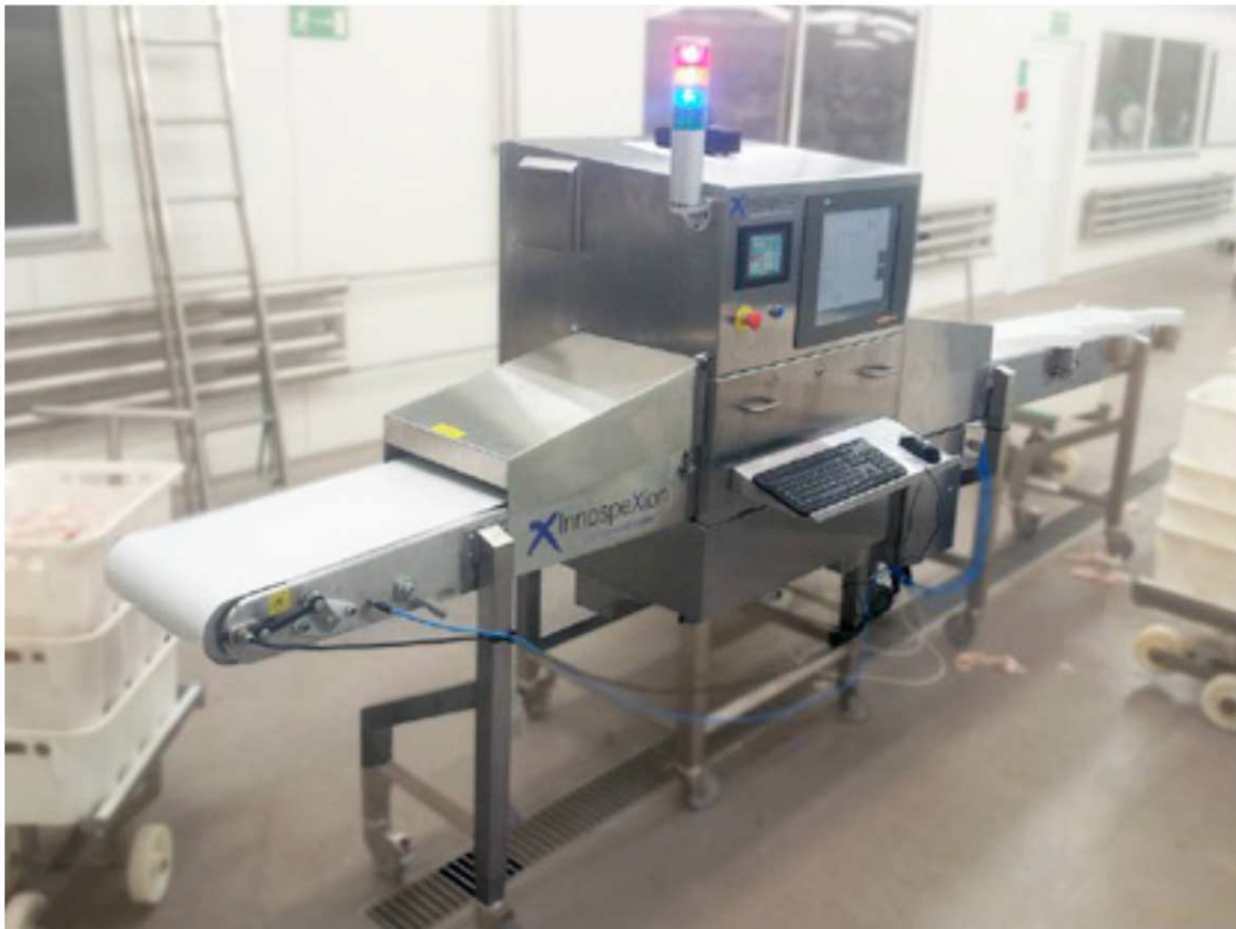
At Espersen in Poland, the X-ray technology was initially evaluated based on off-line usage. Experience shows that the technology is much more reliable and robust than human inspection. Today, all relevant products are inspected using X-ray systems, in an in-line arrangement.
