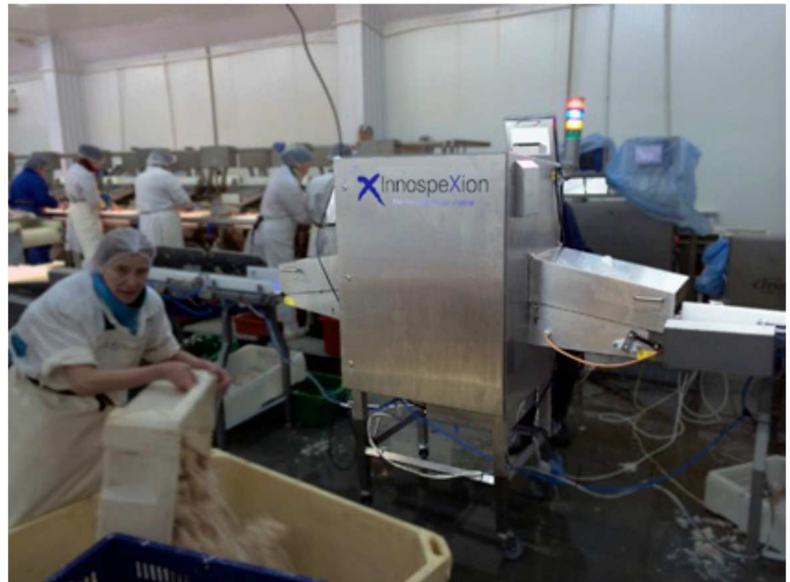
Overview of an application similar to Espersen, but involving different production line set-up. Here, the X-ray system is used for control of the quality of the work performed on the filleting line, as part of a task of improving the overall quality and significantly reducing the bone content by an iterative learning procedure based on the X-ray system bone detection
