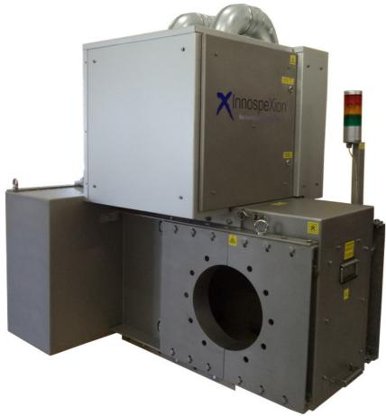
1. Dual view X-ray system with integrated climate control for placement on spool rig pipe in northern Norway. Pipe internal diameter 200 mm. Imaging up to 10 m/s.
