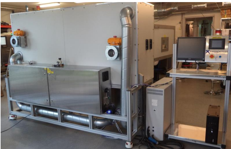
Fig. 6. Linear core analysis X-ray scanner for horizontal cylindrical core, up to 1 m long, placed in a high stability oven (100-120 deg C). The system is based on a high stability X-ray source, a scintillation detector, and a high sensitivity high speed X-ray image detector, all positioned on a linear guide. Based on references placed at the end of the core holder, the 2 or 3-phase composition is calculated following each scan. Scan time for a core of 60 cm is about 3-10 minutes, depending on detector aperture and integration time at each measurement point. Flow imaging across the entire core can be performed in 10 s. The system integrates a control PC with acquisition and processing hard- and software, coolers and air-condition unit. Automatic ventilation for CH fume extraction
