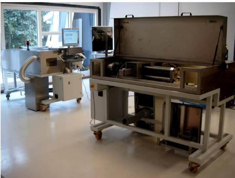
Fig. 4. Linear core analysis X-ray scanner for cylindrical core, up to 1 m long. The system is based on a high stability X-ray source and a scintillation detector positioned on a linear guide. Based on references placed at the end of the core holder, the 2 or 3-phase composition is calculated following each scan. Scan time for a core of 60 cm is about 3-10 minutes, depending on detector aperture and integration time at each measurement point. The system integrates a control PC with acquisition and processing hard- and software, coolers and air-condition unit.
