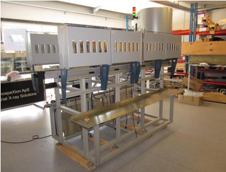
Fig. 5. Cyclic linear X-ray core analysis scanner for short (200 mm) vertically positioned cylindrical cores (up to 48 in total). The system is based on a high stability X-ray source and a scintillation detector positioned on a linear guide. Based on references placed at the end of the core holder, the 2 or 3-phase composition is calculated following each scan. Scan time 0.5-2 minutes per core, depending on detector aperture and integration time at each measurement point. The system is PLC controlled and allows multiple, repetitive measurements over long time.
