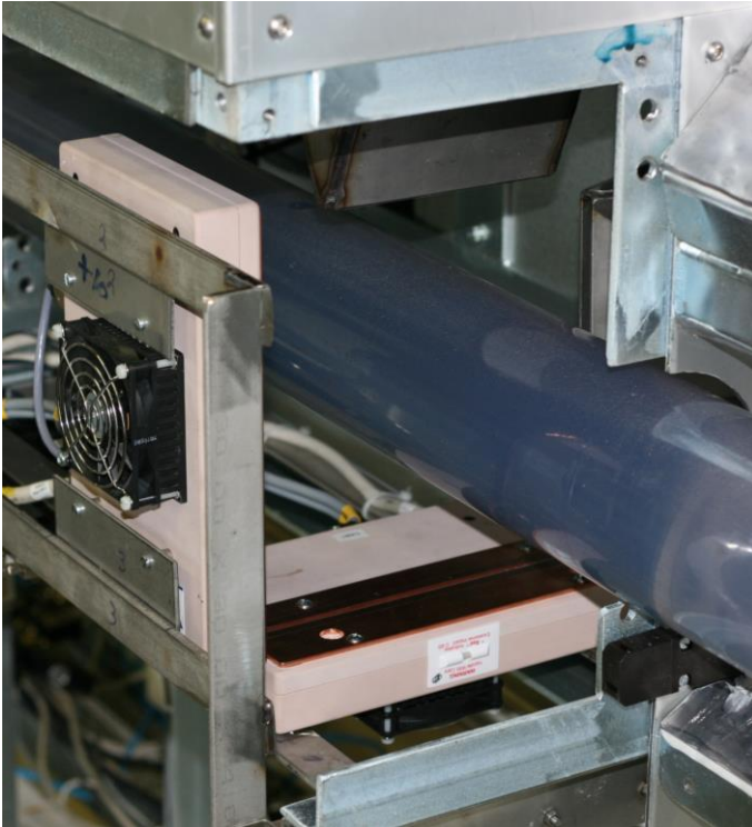
Fig. 8. Detail of a 2-projection imaging system at a 110 mm pipe for Multiphase Flow Measurement. The pipework is stainless steel, but the X-ray imaging window is typically plastic or CFRP. X-ray imaging can take place at flow speed over 10 m/s.
