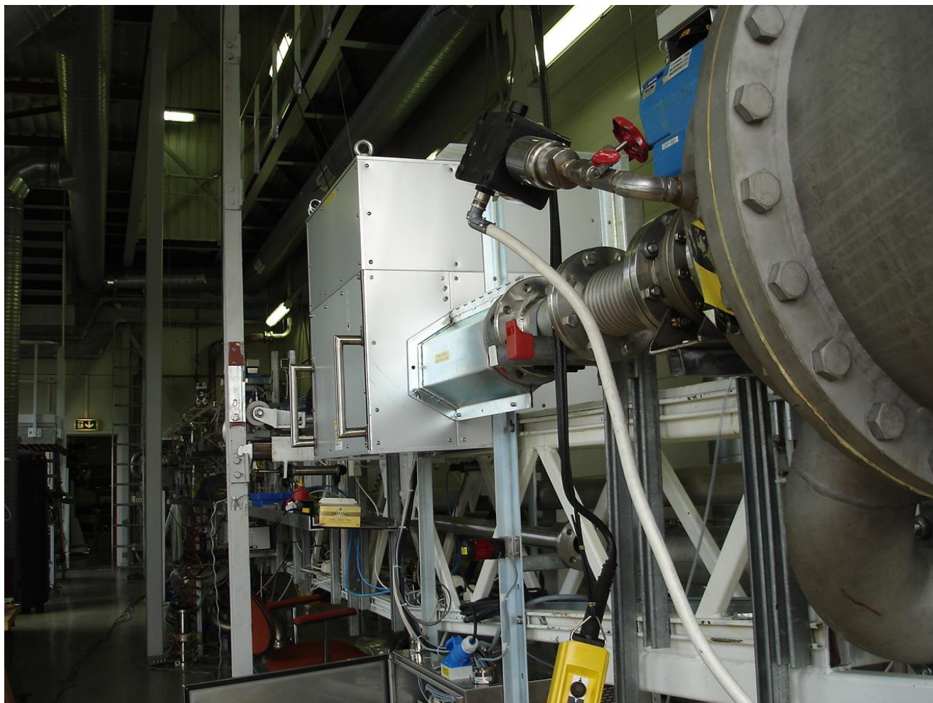
Fig. 7. X-ray system for Multiphase Flow Measurement mounted on pipe spool rig (20 m) in laboratory, for positioning between horizontal and vertical. Dual source-detector configuration (at 90 degrees). Remote control and image capture station. 110 mm diameter pipe.
