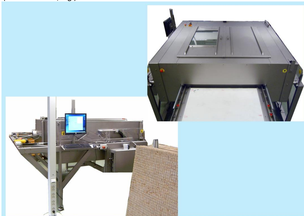
Fig. 2. The InnospeXion rock slab scanner integrates fast X-ray image scanning and slow (but precise) point measurements with single crystal detector with multi-channel analyzer.
