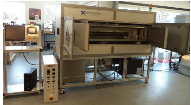
Fig. 6. Linear core analysis X-ray scanner for horizontal cylindrical core, up to 1 m long, placed in a high stability oven (100-120 deg C). The system is based on a high stability X-ray source, a scintillation detector, and a high sensitivity high speed X-ray image detector, all positioned on a linear guide. Based on references placed at the end of the core holder, the 2 or 3-phase composition is calculated following each scan. Scan time for a core of 60 cm is about 3-10 minutes, depending on detector aperture and integration time at each measurement point. Flow imaging across the entire core can be performed in 10 s. The system integrates a control PC with acquisition and processing hard- and software, coolers and air-condition unit. Automatic ventilation for CH fume extraction
