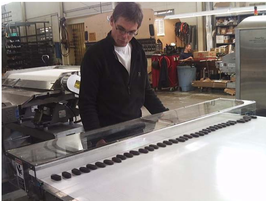
Fig. 5. Chocolate bar alignment prior to reject tests with 38 chocolate lanes across a 1600 mm conveyor width of a chocolate X-ray inspection system .
