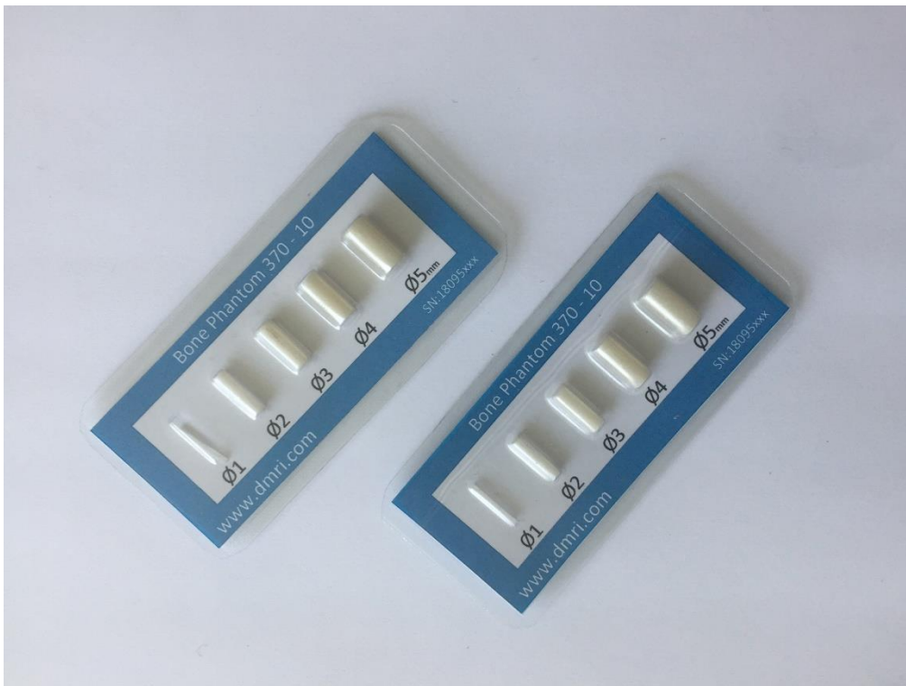
Fig. 3. Test samples with artificial bone pieces in the form of cylindrical samples 10 mm long and with diameters from 1 to 5 mm, all with 370 HU value (average chicken bone). Test samples provided by DMRI.
