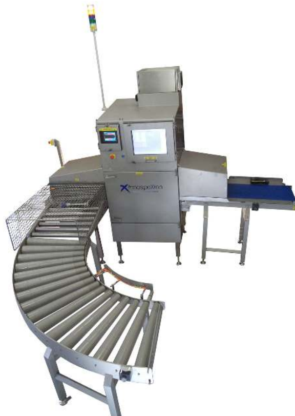
Fig. 4. Layout of the InnospeXion X-ray system designed for large products and packages inspection. Facilitates detection down to 0.2 mm, tailoring to the production line, EHEDG guidelines conformity, proven technology, dedicated software solutions e.g. for cheese internal structure quantification and validation.
