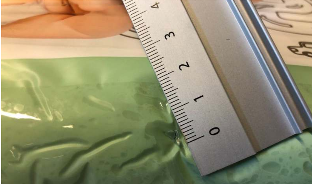
Fig. 4. Image illustrating the inspected package of disposable baby diapers with a smaller glass fragment during the second round of tests (4mm long), which has been positioned towards the bottom and place under the diapers package.
